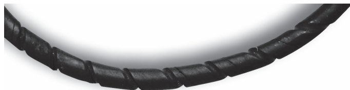
Fig. 9.10 Twisted O-ring with spiral marking
