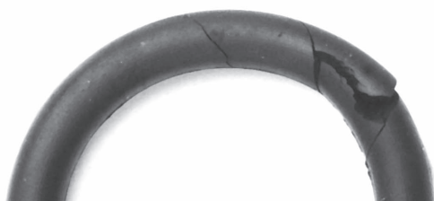
Fig. 9.11 Twisted O-ring with spiral cuts in surface
