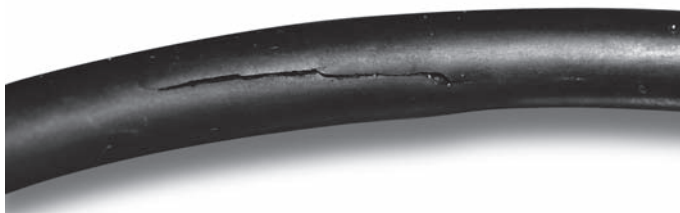
Fig. 9.12 O-ring damaged by explosive decompression
