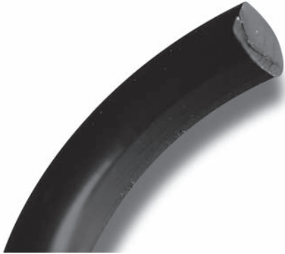
Fig. 913 Wear is seen as flattening of O-ring on one side
