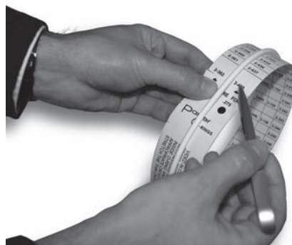
Identification of the O-ring size using the measuring band
