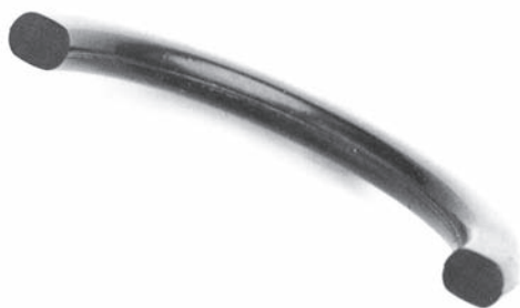
Fig. 9.9 Characteristic compression set. High deformation
